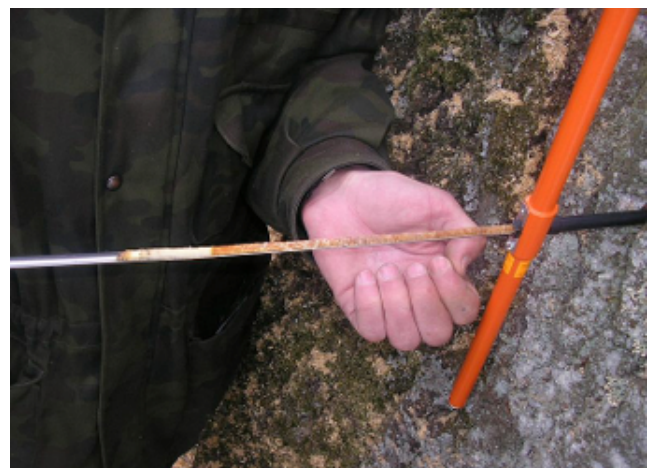
Figure 3: removing the extractor tray and tree core.
